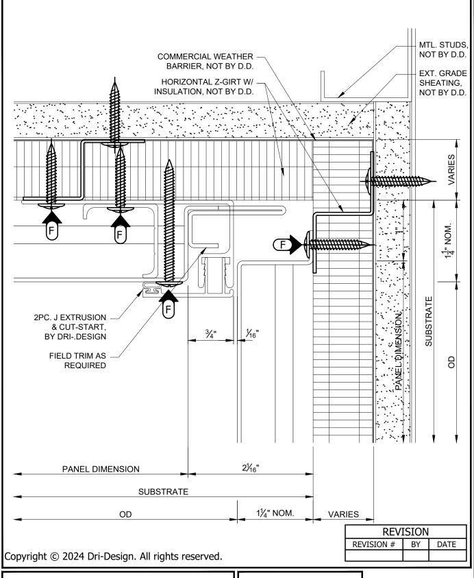
SOFFIT TO VERTICAL WALL DETAIL (EXTRUSION)
