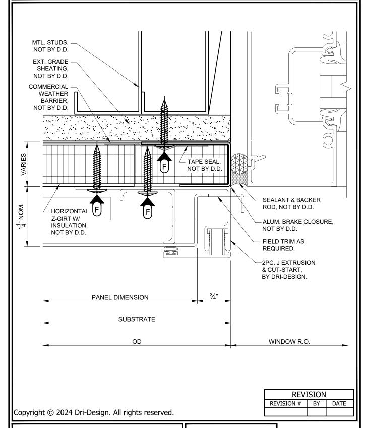
JAMB DETAIL AT STOREFRONT (EXTRUSION) DETAIL #: DD STANDARD TYP. EXT. W. JAMB
